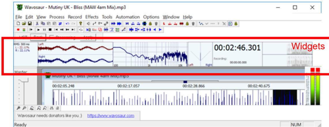
RMS: shows in real time root mean square value of output signal
